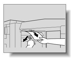
**10** Open the transport guide, and then pull out any misfed paper in the transport section.
